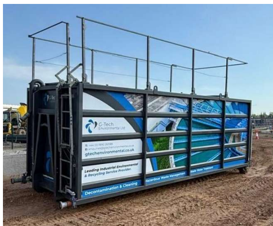
De-Watering Box with handrails raised for access to top of equipment
